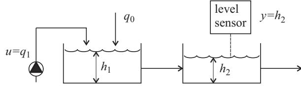
In the operating point the transfer function from the control signal  $u$  to the level  $h_1$  in the first tank is given by
