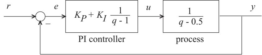
The idea in this problem is to show how PI controller parameters can be determined by state feedback optimization.
