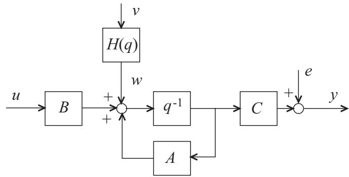
Neither  $w$  nor  $v$  can be measured online to be used in a feed forward control. However, from separate system identification experiments the pulse transfer operator  $H$  from  $v$  to  $w$  has been determined to be
