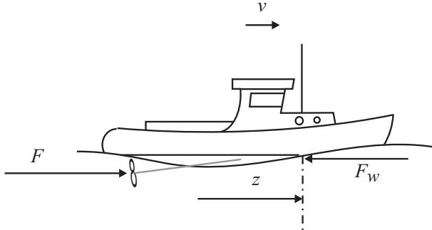
Let the boat position be  $z(t)$  [m], the boat speed be  $v(t)$  [m/s] and the propulsion force be  $F(t)$  [N]. We may assume all friction forces together be related to the speed according to
